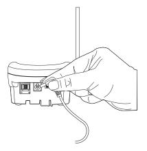
Place the AC Adapter cord inside the molded channel.
